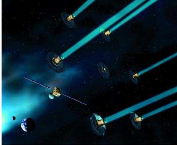
Figure 1.1: Schema of the Darwin formation with six telescopes. The telescopes are located in the vertices of an hexagon and the collector on the centroid of this hexagon.
