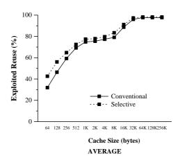
**Figure 4.7.** Percentage of reuse exploited with a selective cache, varying the cache size and compared with a conventional cache.
