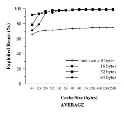
Figure 3.8. Percentage of reuse exploited with a varying cache size without interferences.
