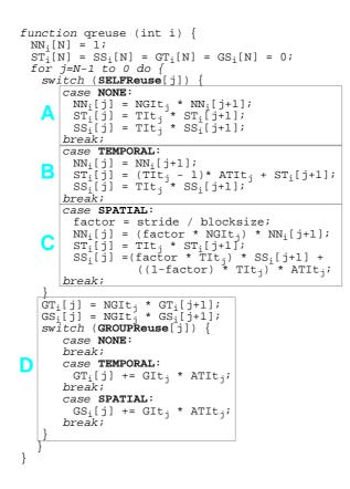
Figure 2.2. Algorithm to quantify intrinsic reuse
