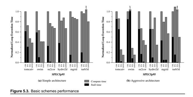
An approach to reduce the processor stall is to insert a prefetch instruction for every memory operation. Such instructions are scheduled at a distance equal to the cache-miss latency from the actual memory references. This scheme will be called *insert prefetch always* (IPA). However, this scheme may result in an increase in the number of operations (due to prefetch instructions but also to some additional spill code) and therefore, it may require an *II* higher than the previous approaches.
