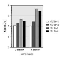
Figure 6.9. Speedup of clustered architectures with respect the unified one (bus latency=1 cycle)
