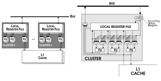
Figure 6.1. VLIW clustered architecture and detailed architecture of a single cluster
