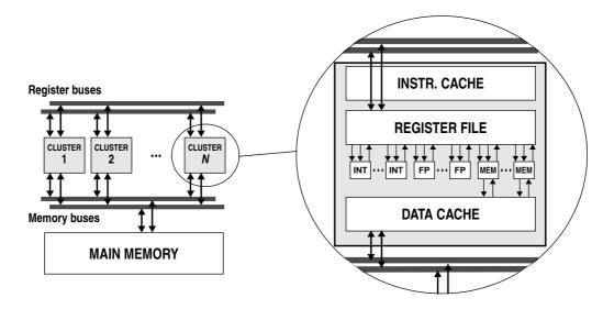
Figure 6.11. Microarchitectures of a MultiVLIWProcessor
