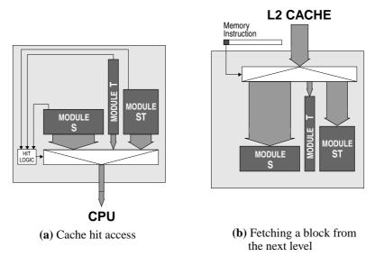
Figure 4.8. Hardware architecture of the LSMCache
