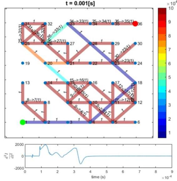
**Fig. 4** Visualization of the simulation results after 0.001s for an SPP computation concerning the search of a path from node 1 to 36 in a random directed graph defined on a  $6 \times 6$  grid, while applying a voltage ramp rising from 0 to 100V in 1ms. Memristors were simulated using the memristor model of [19] with  $[R_{ON}, R_{OFF}] = [2, 200]K\Omega$  (see description in section 3). At the bottom, the evolution of the 2<sup>nd</sup> time derivative of the current is shown.
