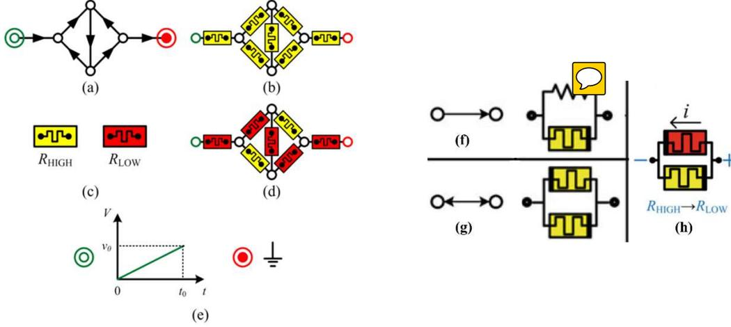
**Fig. 1** (a, b) Example of a directed graph mapped to a memristive network. (c, d) The solution to the SPP marked with memristive components shown in red color. (e) The input voltage applied to the SRC and the ground applied to the DST node. (f, g) Mapping correspondence for directed and undirected graph edges according to [15]. (h) Polarity-independent switching of antiparallel memristors emulating an undirected edge of a graph.
