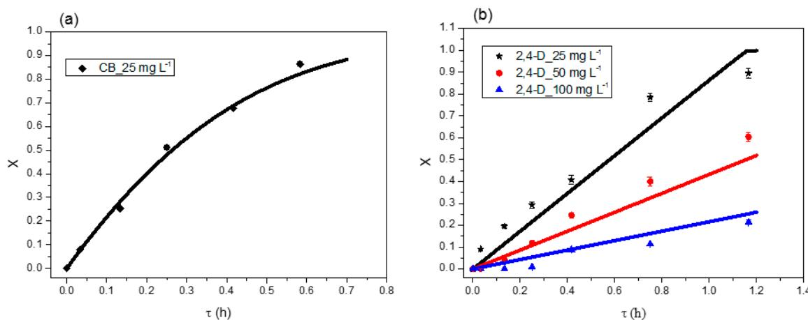
**Figure 6.** Kinetic modelling of CB (a) and 2,4-D (b) biodegradation in USPBRs. Lines represent fitting to the Michaelis-Menten model ( $T = 35^{\circ}\text{C}$ ).
