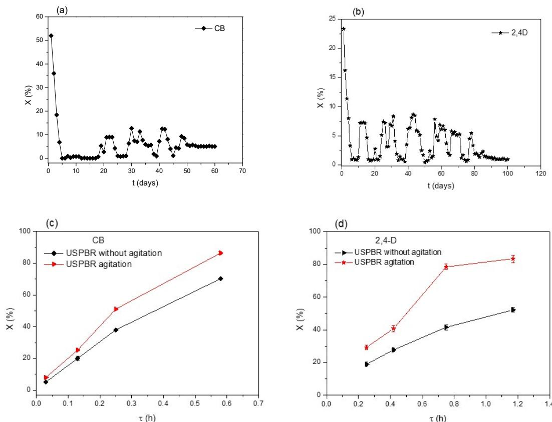
**Figure 4.** (a,b) Acclimatization and stabilization period of USPBRs for CB ( $[CB]_{in} = 25 \text{ mg L}^{-1}$ ,  $T = 35^\circ\text{C}$ ,  $\tau = 0.033 \text{ h}$ ) and 2,4-D ( $[2,4-\text{D}]_{in} = 100 \text{ mg L}^{-1}$ ,  $T = 35^\circ\text{C}$ ,  $\tau = 0.033 \text{ h}$ ). (c,d) Performance of USPBRs at different space times for CB and 2,4D ( $[CB]_{in}$  or  $[2,4-\text{D}]_{in} = 25 \text{ mg L}^{-1}$ ,  $T = 35^\circ\text{C}$ ), with and without stirring.
