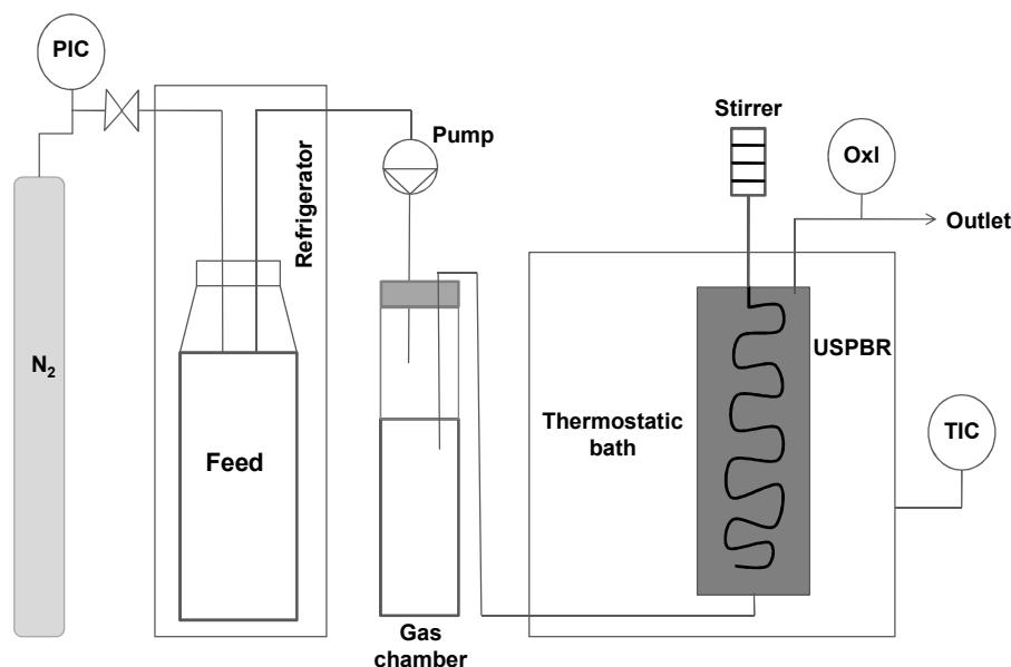
**Figure 2.** USPBR experimental setup.
