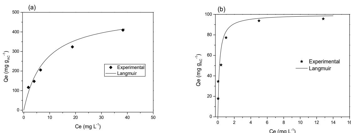
**Figure 3.** Equilibrium adsorption isotherms of CB (a) and 2,4-D (b) over activated carbon ( $35^\circ\text{C}$ ). Symbols represent experimental data and lines are fitting to the Langmuir equation.
