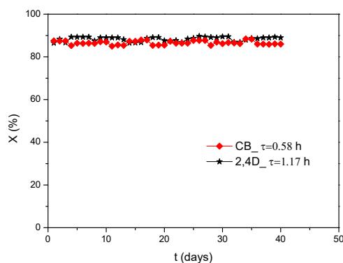
**Figure 5.** Stability of the USPBR system during long operation periods. ( $[\text{CB}]_{\text{in}} \text{ or } [\text{2,4-D}]_{\text{in}} = 25 \text{ mg L}^{-1}$ ,  $T = 35^\circ\text{C}$ ).
