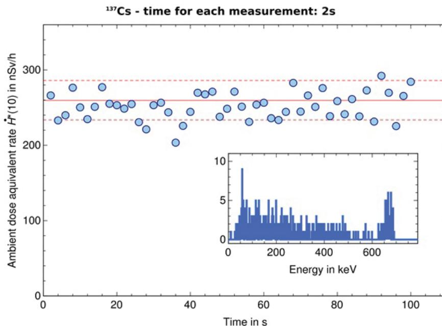
**Figure 2** Test results from a measuring campaign on PTB’s premises, where an uncollimated free field irradiation facility was operated. This facility can also be used for the simulation of a by-passing radioactive plume (6). The spectra (inset) are recorded every 2 s and the average dose rate during these 2 s is calculated for each spectrum individually. Most measured dose rate values lie in a 10% range around the reference value of 259 nSv/h indicated by the dashed lines
