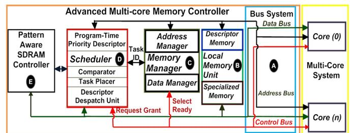
Fig. 1. Architecture of the Advanced Multi-core Memory Controller
