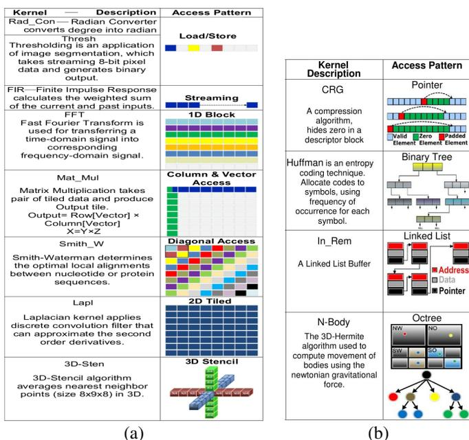
Fig. 3. Application Kernels: (a) Regular Access Pattern (b) Irregular Access Pattern
