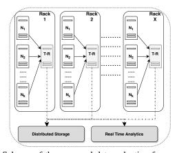
Fig. 1: Schema of the proposed data reduction framework for data centers. Each rack in the data center hosts a Telemetry Reductor (T-R) component which continuously collects the telemetry data from each computing node, then performs data reduction before transmitting it to storage and real-time analytic systems.
