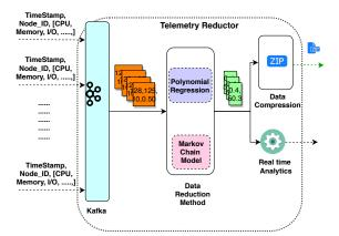
Fig. 2: Telemetry Reductor process the incoming telemetry streams from computing nodes using Kafka and data reduction method. The output of the Telemetry Reductor can be used to store or provide input to other real-time analytics systems.
