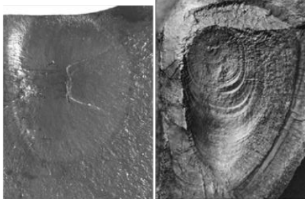
Figure 3: Characteristics of tooth flank fracture, fisheye of constant loading [7], fisheye with beachmarks due to the crack growth under varying loading [1]
