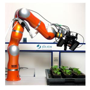
Figure 1: Robot gardener used in the European project GARNICS. A black-and-white 5 MP camera with infrared filter and required illumination devices were mounted on a lightweight KUKA LBR4 robot arm. For each tobacco plant the robot arm captured a stereo image pair from a top view at every hour.
