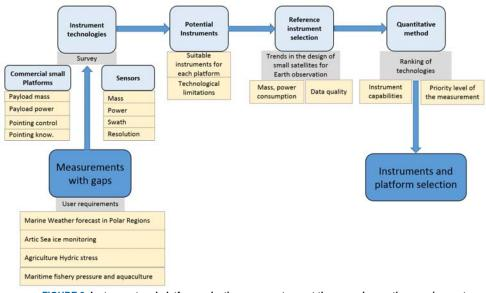
FIGURE 3. Instrument and platform selection process to meet the user observation requirements.
