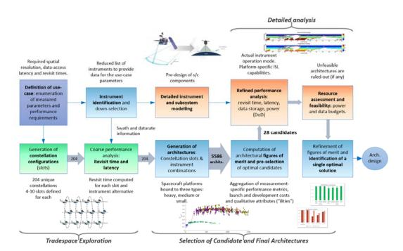
FIGURE 2. Graphical explanation of the Systems Architecture Study to select the optimum configuration.
