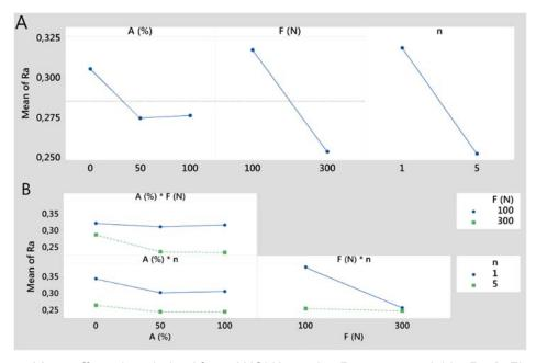
**Figure 8.** Mean effect plots derived from ANOVA results. Response variable: R<sub>t</sub>. **A.** First order effects. **B.** Second order interactions among factors.
