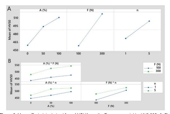
**Figure 8.** Mean effect plots derived from ANOVA results. Response variable: HV0.005. **A.** First order effects. **B.** Second order interactions among factors.
