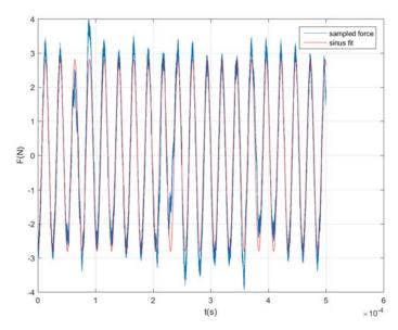
Figure 4. Registered signal and sinus fit for 600 N and a 100% A.
