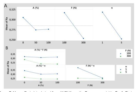
**Figure 7.** Mean effect plots derived from ANOVA results. Response variable: R<sub>a</sub>. **A.** First order effects. **B.** Second order interactions among factors.
