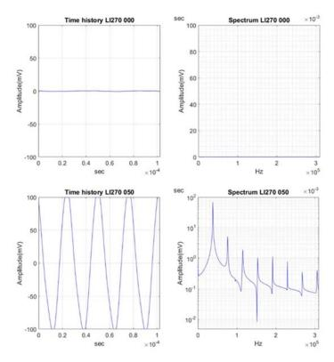
**Figure 3.** Registered signals for the burnishing line tests applying a 270 N preload, and 50% amplitude VABB and no vibration.
