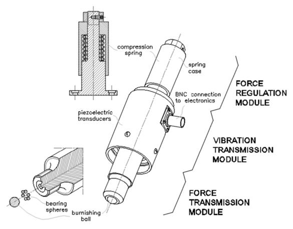
Figure 1. General scheme of the proposed design for the VABB tool.
