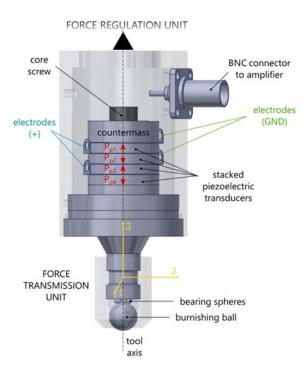
**Figure 2.** Detail of the piezoelectric stack inside the vibrations transmission unit joint to the force transmission unit.
