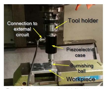
Figure 5. Experimental setup to perform the ball burnishing tests.
