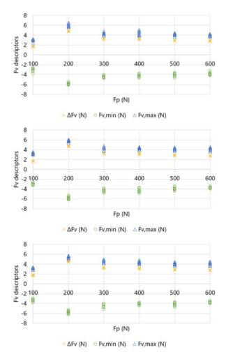
Figure 5. Half cycle vibratory force variation and extreme values for different preload levels.
