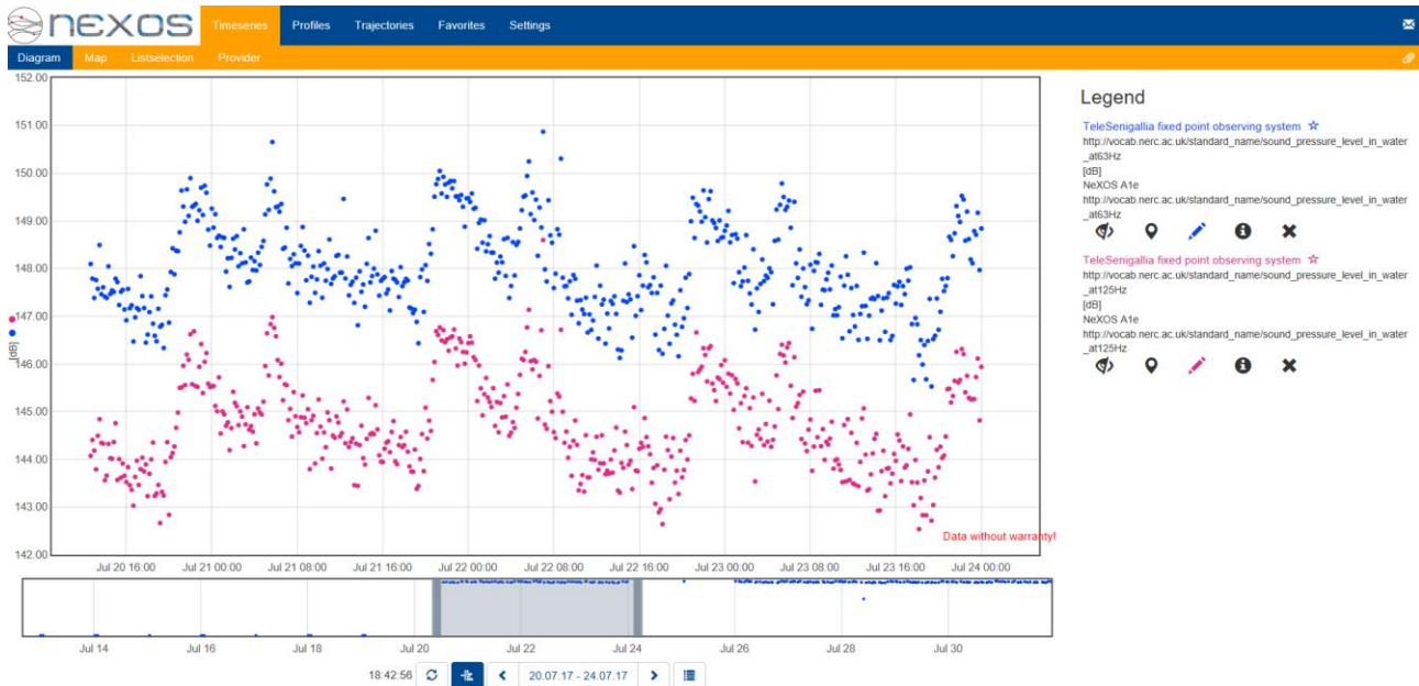
Figure 18 Time series of RMS sound pressure level in water for MSFD Indicator 11.2.1 (at 63 Hz - blue and 125 Hz - red) in the TeleSenigallia site, starting from July 20 until July 24, 2017. The x-axis is date and time
