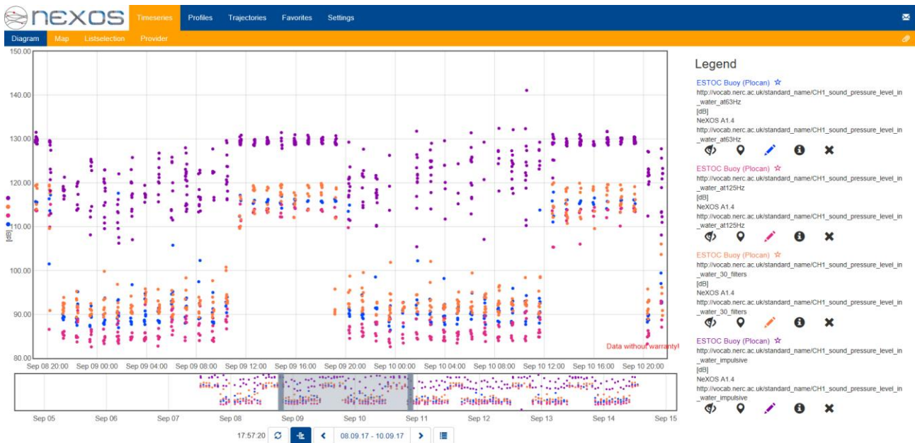
Figure 16 Time series of RMS sound pressure level in water for MSFD Indicator 11.1.1 (purple), MSFD Indicator 11.2.1 (at 63 Hz - blue and 125 Hz - red) and Extended MSFD Indicator 11.2.1 (orange), in the ESTOC site, starting from September 8 until September 11, 2017. The x-axis is time.
