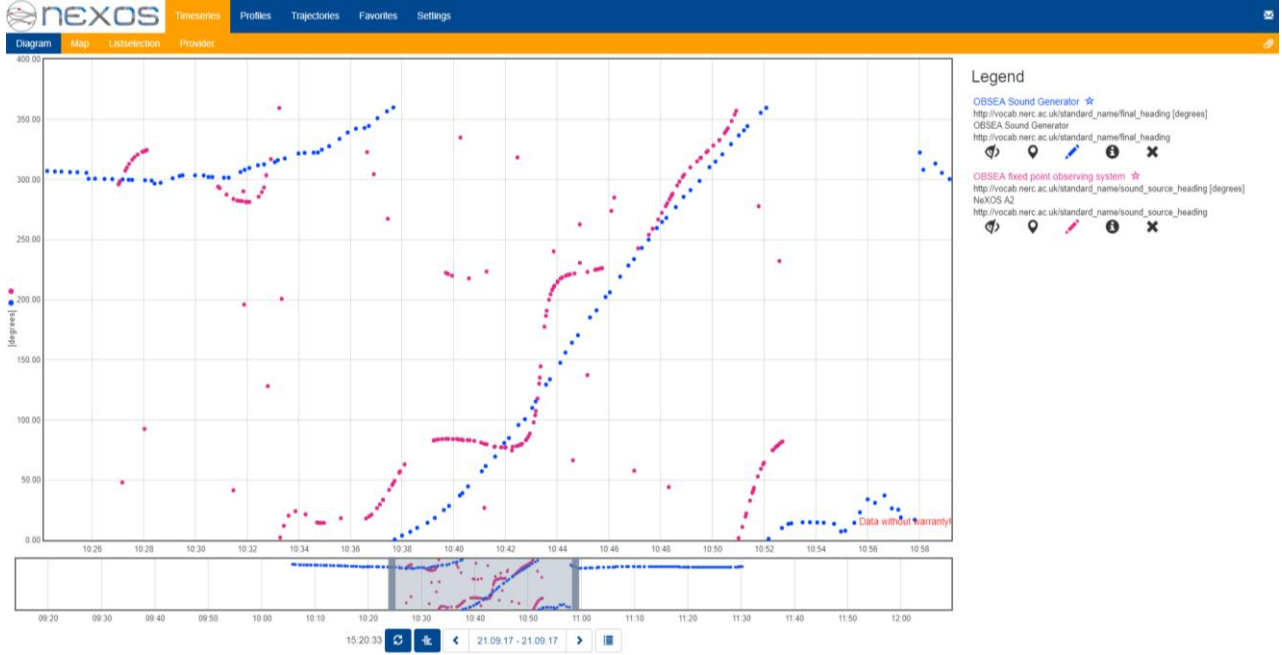
Figure 20 A2 DOA vs GPS-measured of boat location, delivered to NeXOS SOS and viewed in the NeXOS SWE viewer
