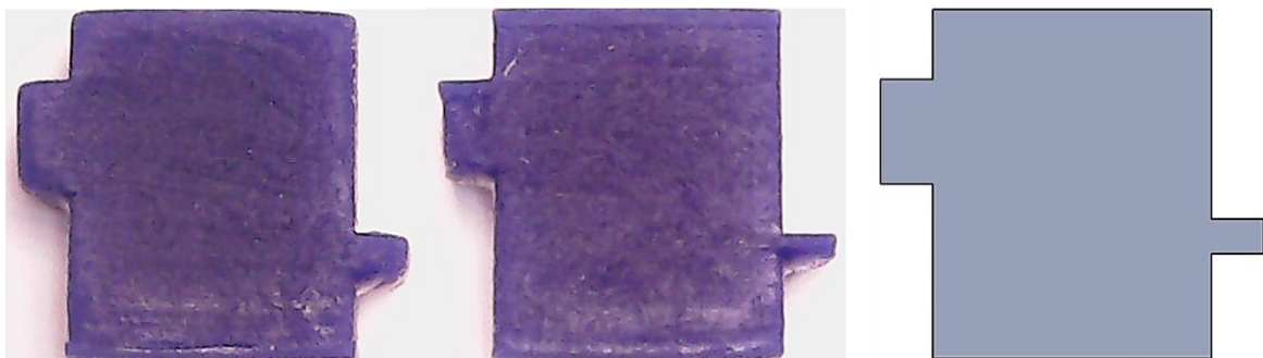
Figure 19 - Case 2 parts obtained without (a) and with the optimisation procedure (b). Objective part (c). A higher dimensional accuracy is obtained in optimised parts.
