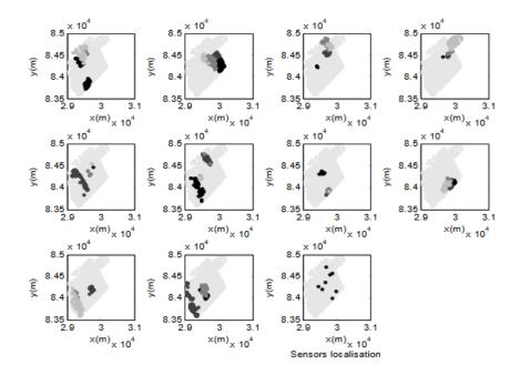
Figure 6. Groups of nodes with the same leakage signature with 8 sensors and placement of sensors
