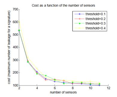
Figure 5. Evolution of the cost function (maximum size of group of possible leaky nodes) depending on the number of sensors and threshold.
