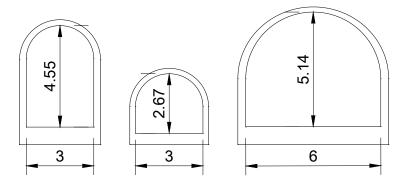
Figure 5. Drains with cast-in-place concrete arch analysed in the case study.
