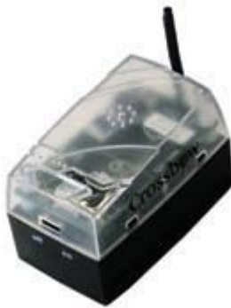
Figura 2.2 Nodo Crossbow MPR2600
