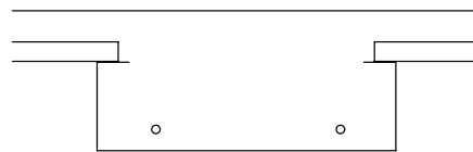
Figure 3.2 Finnish system of light steel composite construction
