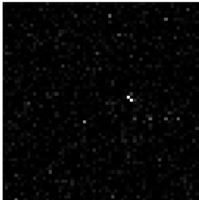
Fig. 8. Result of the application of the spatial correlation to the four components presented in Fig. 7. The presence of the ship is enhanced, whereas background noise is reduced.
