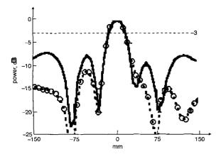
Fig. 3 Predicted and measured power distribution for 126 mm focal length array at  $10~\mathrm{GHz}$
