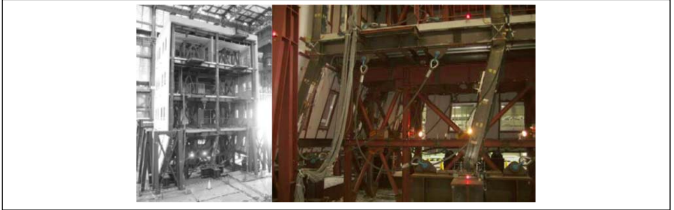
Figure 4. Structure collapsed after the 100% Takatori record
