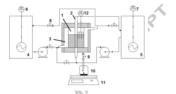
Fig. 1. Experimental set up for block freeze concentration
