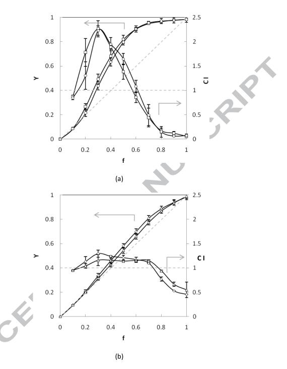
Fig. 7. Effect of heating temperature on solute yield and the concentration index. a) Test 2,  $T_H = 20 \ ^{\circ}C (\Box)$ ; Test 4,  $T_H = 40 \ ^{\circ}C (\circ)$ ; b) Test 10,  $T_H = 20 \ ^{\circ}C (\diamond)$ ; Test 12,  $T_H = 40 \ ^{\circ}C (\Delta)$
