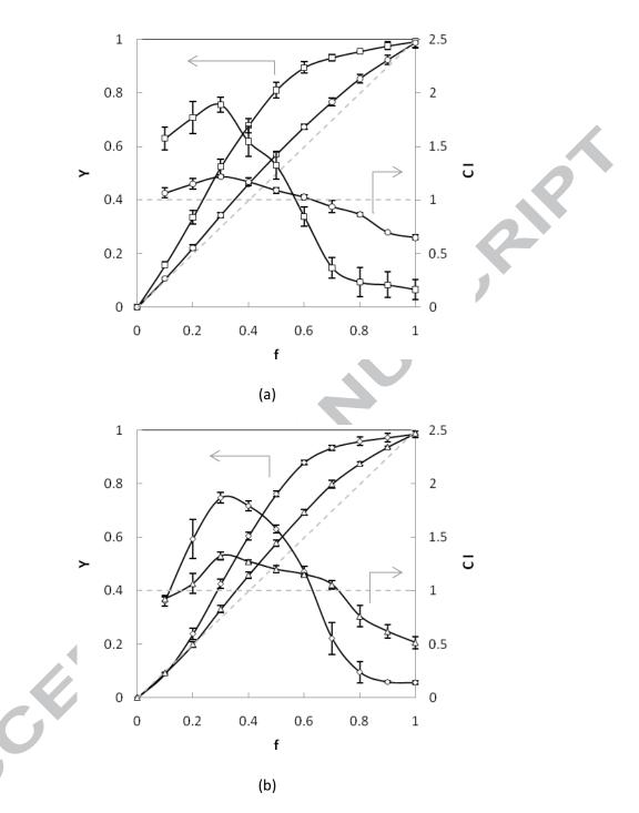
Fig. 4. Effect of coffee mass fraction on solute yield and the concentration index. a) Test 5,  $X_S = 5\%$  ( $\Box$ ); Test 13,  $X_S = 15\%$  ( $\circ$ ); b) Test 6,  $X_S = 5\%$  ( $\diamond$ ); Test 14,  $X_S = 15\%$  ( $\Delta$ )
