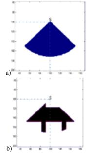
4. a) Generated area of 90°, formed by the combination of the beam generated by the sonar located on the X = Y = 100m, b) Response obtained by the SDO
