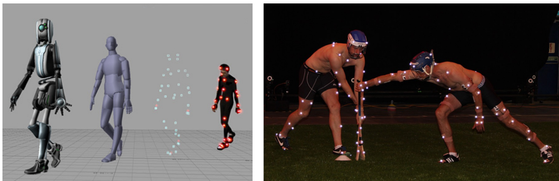
Figure 1.1: Two scenarios where the non-rigid reconstruction could be useful. On the left there is a person being tracked with several points marked in red, which lately those points have been transferred to a virtual space overlapping a robot shape which follows the same actions the actor performed. On the right two field hockey players are being tracked to monitor their activity and evaluate the performance [1]. Currently, these models are acquired with complex and expensive motion capture systems, based on multi-camera systems. In contrast, we propose a method that only uses a monocular camera.
