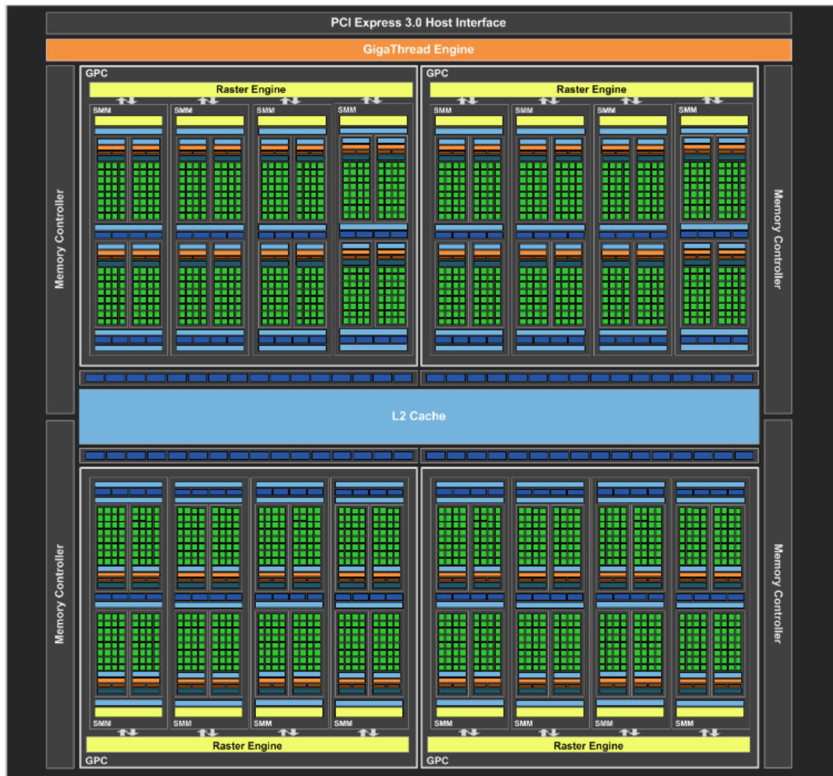
Figure 10.4: GM204 Full chip block diagram [30]
