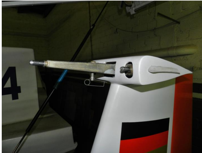
Figure 5. Fixed part of the tail, notice that the bar enables the aircraft to pitch.
