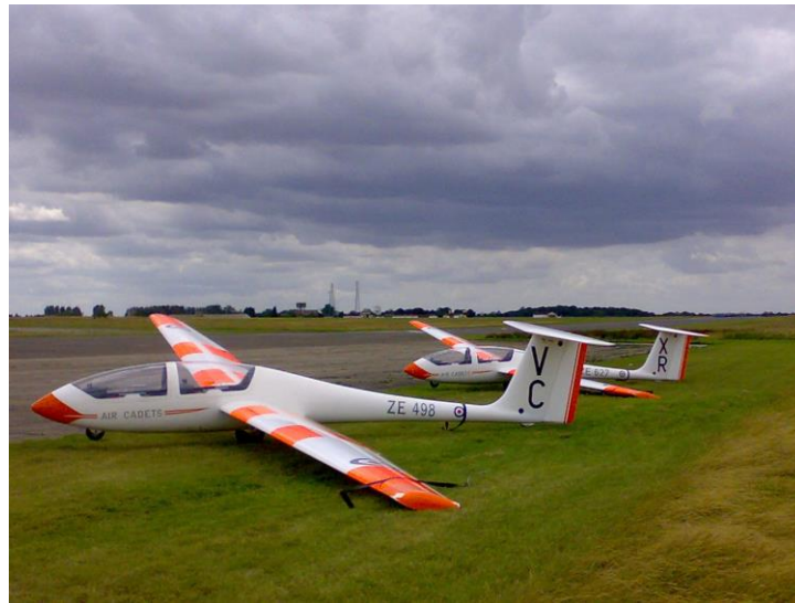
Figure 2. The wing tip must touch the ground for the rest position.
