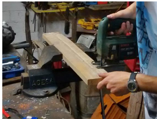
Figure 25. Cutting off of the main piece from a wood strip
