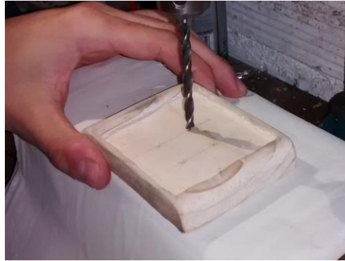
Figure 27. Drilling of the first big hole.
