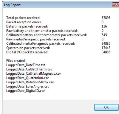
Figure 14: x-IMU GUI data logger report
