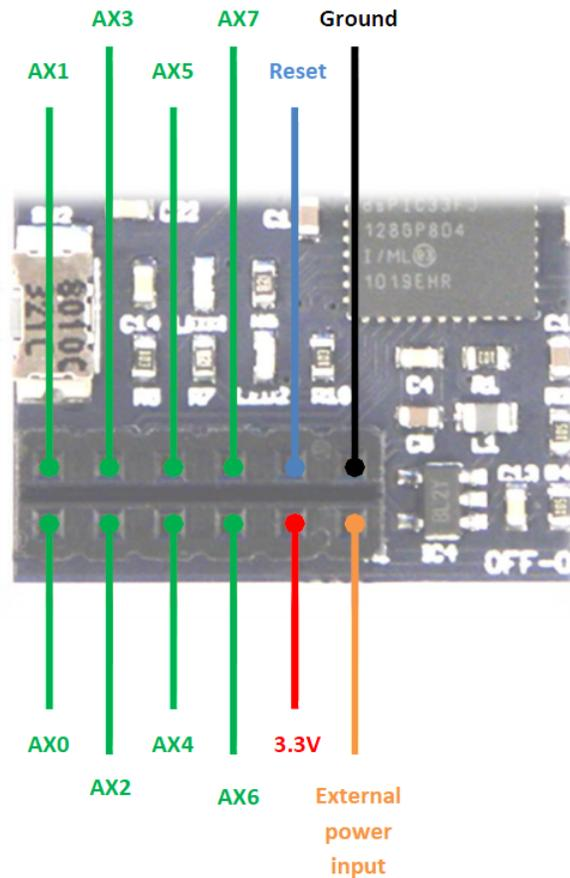
Figure 23: Auxiliary port pins
