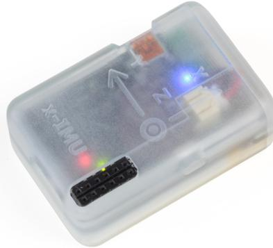
Figure 1: x-IMU and battery in plastic housing
