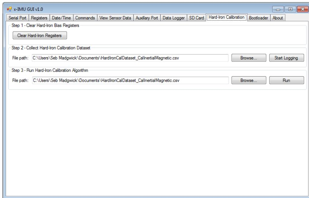
Figure 22: x-IMU GUI hard-iron calibration tab page
