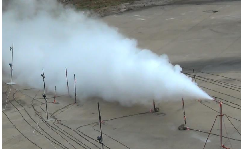
Figure 33 - Image of trial P25_2, showing the release point and masts; at 40 s from the beginning of the release and release rate of 0.17 \text{ kg}\cdot\text{s}^{-1} .
