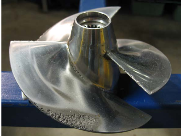
Figure 1.1: Cavitation damage in a propeller.
