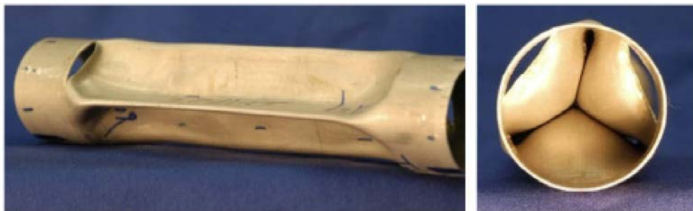
Figure 4.19: Experimental results for third buckling mode [3]
