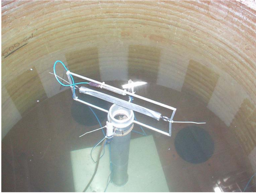
Figure 5.5: Aluminum cylinder filled with air and submerged into the water tank. Sensors are put in 10.16 cm from the center of the cylinder.
