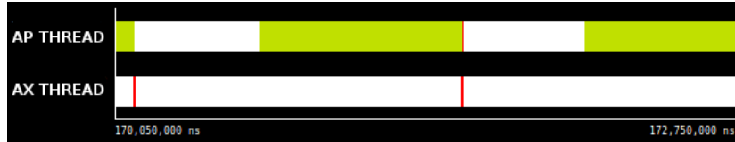
(c) Entire transaction: Static allocation of extra resources to auxiliary threads throughout the whole transaction.
