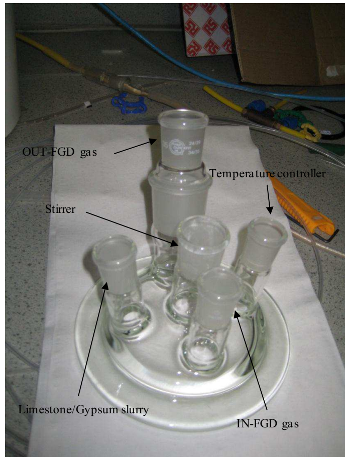
Figure 2.10. Cap of the FGD reactor.
