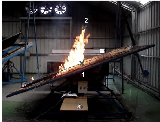
Figure 5.3 Image illustrating points used to measure flame dimensions (upslope fire). The dashed line indicates the central line of the fuel bed and was used as a reference.
