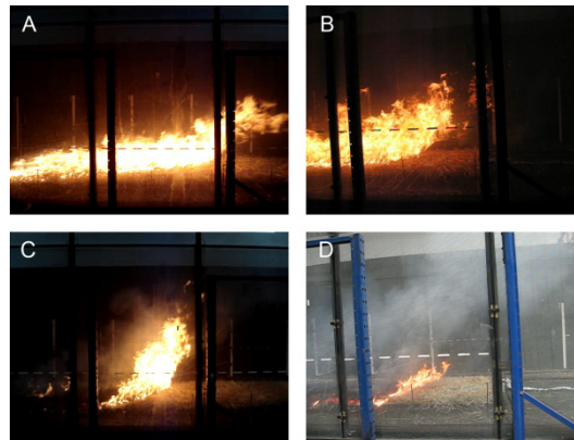
Figure 5.9 Images illustrating different fire situations on a fuel bed of 0.75 \text{ kg m}^{-2} . A) Untreated area; wind velocity: 3.3 \text{ m s}^{-1} ; B) Retardant-treated area; wind velocity: 3.3 \text{ m s}^{-1} ; C) Untreated area; wind velocity: 1.1 \text{ m s}^{-1} ; D) Retardant-treated area; wind velocity: 1.1 \text{ m s}^{-1} .
