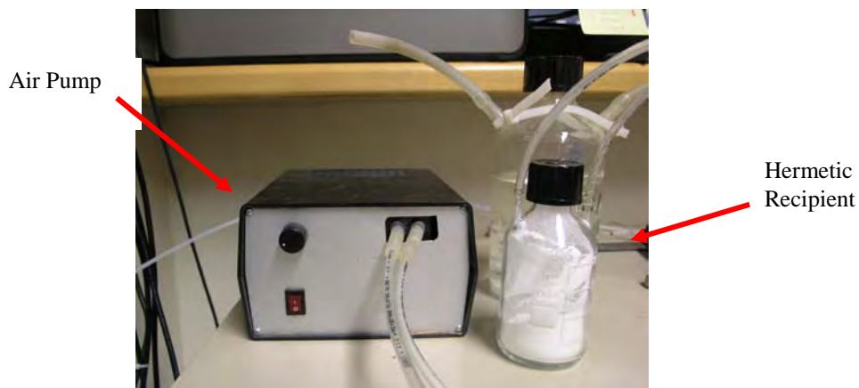
Figure 4.3: Description of vapour forced convection circuit system.
