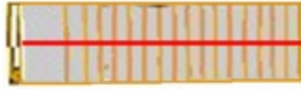
Figure 5.4. Illustration of the analysis line (here red) for the extraction of the fracture mechanics parameters. Every orange line defines a crack front. In this case there are 17 crack fronts
