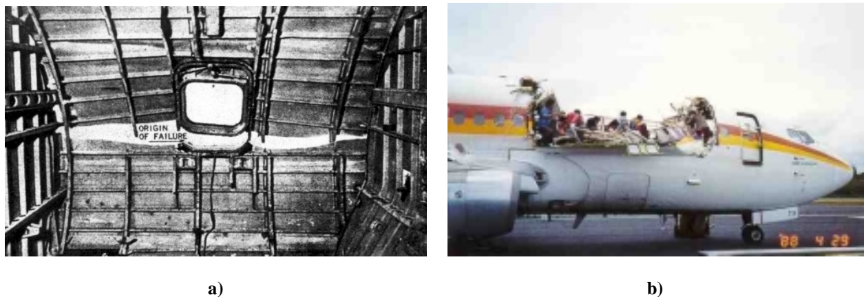
Figure 2.23. Failure of a) Comet transport jet aircraft from fatigue. b) Aloha Flight 243 in which the airplane lost a large section of its upper fuselage due to MSD
