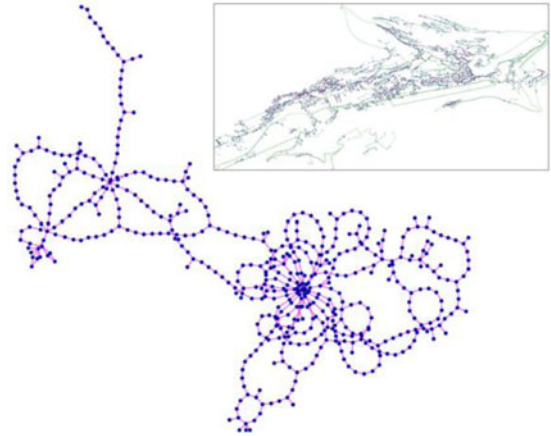
Fig. 1. Example of an urban power distribution network. Red lines are power cables (i.e., edges) and blue dots are substations (i.e., nodes). Inset: spatial graph representation of the same network.
