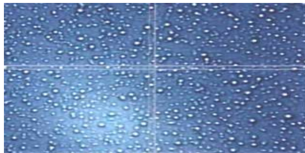
FIGURE 1. -PHOTOMICROGRAPH OF WATER PARTICLES IN A DIESEL OIL EMULSION
