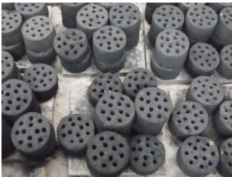
Briquettes are made out of wood, leaves, twigs, branches and any other kinds of agricultural and forestry residue. These are converted to char by carbonising in a charring drum, grinding into powder, mixing with bentonite clay and water, then filled compactly into a mould and dried in the sun for 2 or more days.
