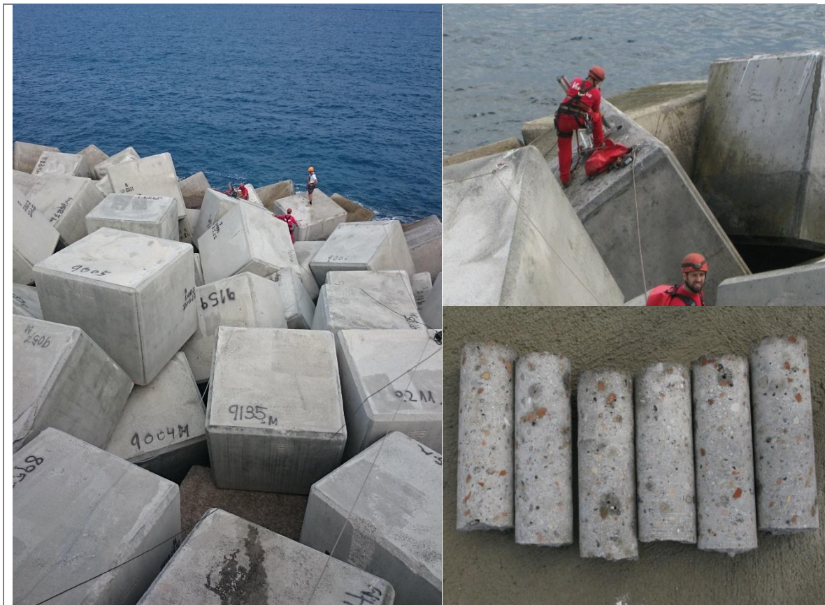
Figure 3. Core extraction process of the blocks after 1 year of being exposed to a sea environment
