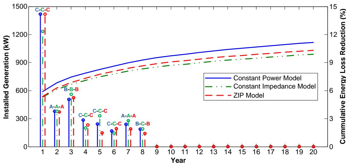
Figure 4. Sequential connection of optimum rated PV generators – Conventional Monte Carlo method.
