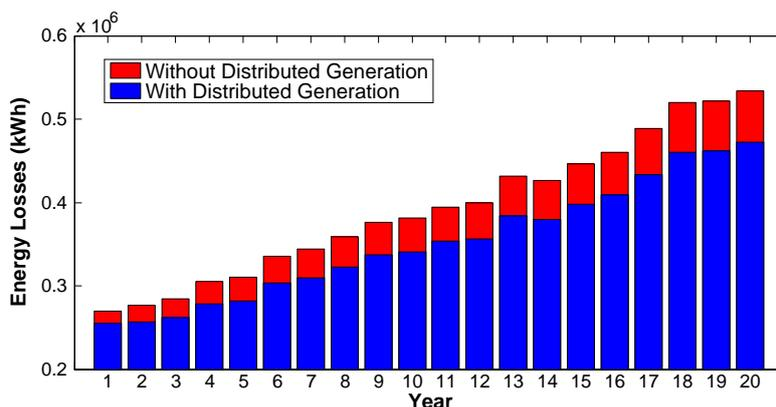
c) Energy losses (without considering substation losses)
