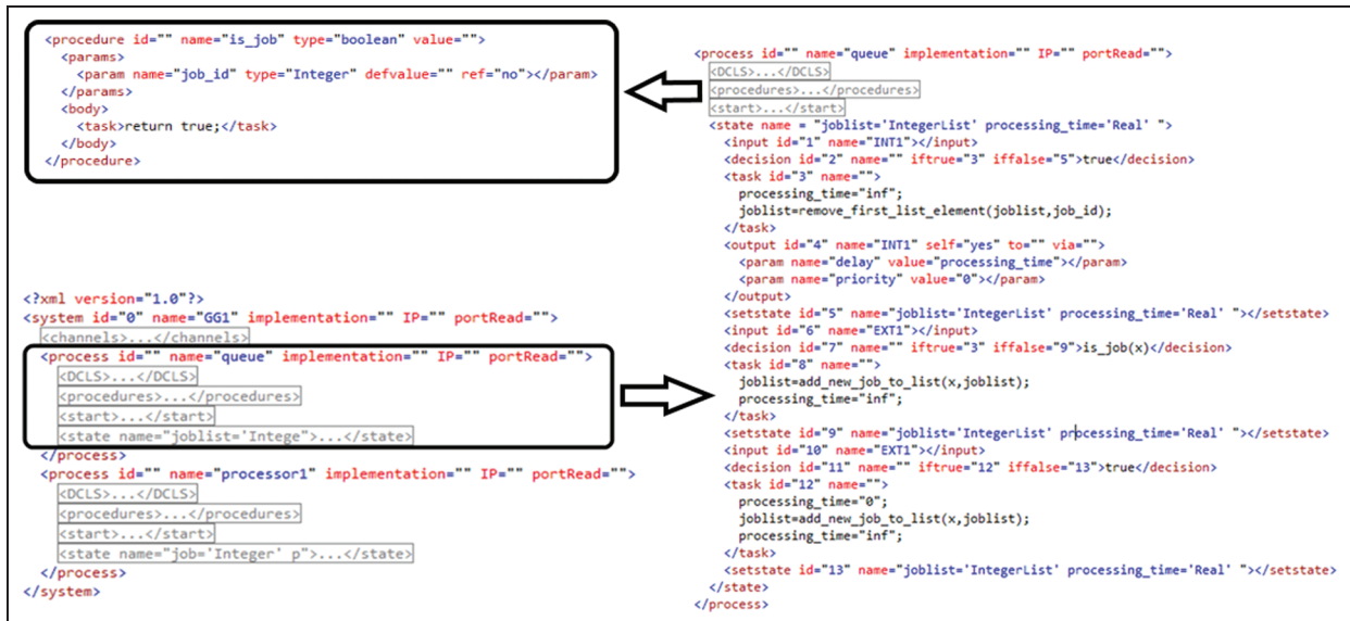
Figure 13. Extensible Markup Language (XML) representation of the Specification and Description Language model. The detailed XML representation of the PROCESS queue is shown on the right side. The PROCEDURE contains the code that is defined in the procedures Discrete Event System Specification model.
