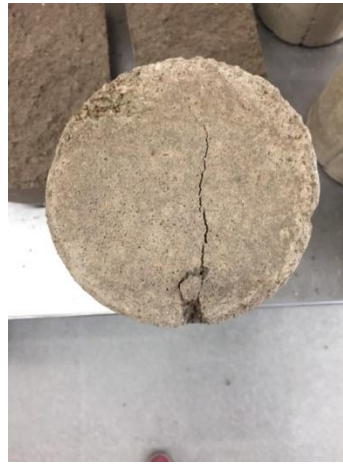
Figure 29. Tensile strength fissure
