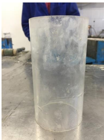
Figure 18. Flow Test cylinder
