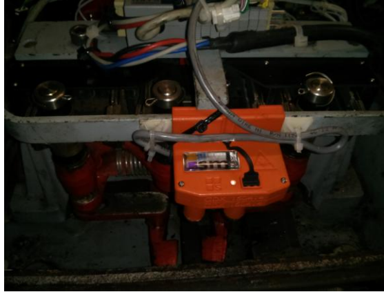
Figure 48. Installed device in a real point machine
