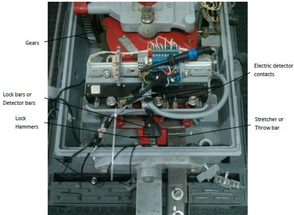
Figure 3. Parts of a real point machine
