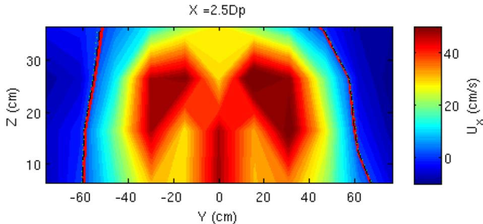
Figure 2. Axial velocity in cm/s at a distance equal to 2.5Dp from the helix plane, when the speed rotation is 400rpm. Red line: Eq. (1); dashed black line: Eq. (2)
