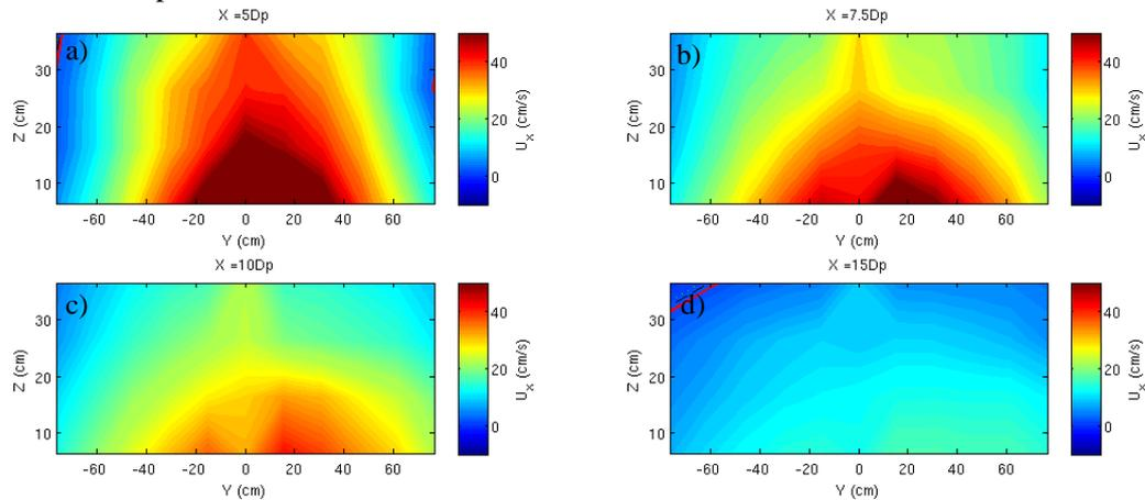
Figure 3. Axial velocity in cm/s at different distances from the helix plane. Speed rotation at 400rpm
