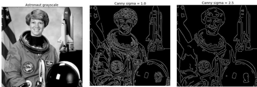
Figure 2.6: The astronaut image with a Canny filter using a gaussian filter of standard deviation of 1.0 and of 2.5.
