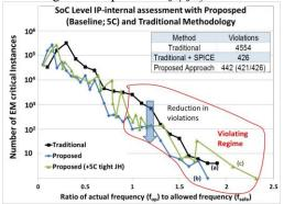
Fig. 8. Distribution plot for a 28nm block (>600K instances), highlighting the number of EM-critical instances for a) traditional, b) proposed and c), proposed method with 5C lower JH. Inset shows reduction in violations.
