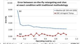
Fig. 6 Validation of retargeting methodology versus SPICE for two conditions, (c) and (e), of Fig. 5.
