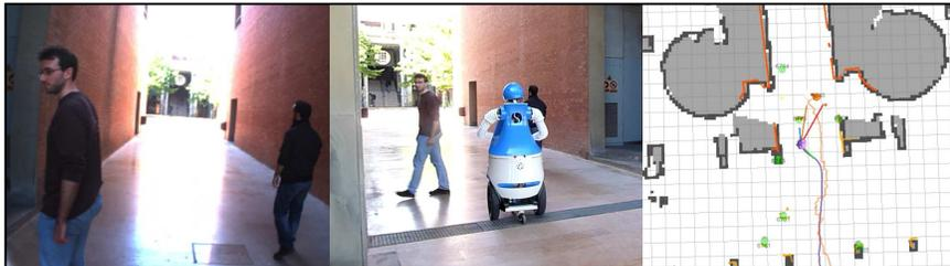
Figure 8: Example of a real robot experiment: Left image corresponds to the robot camera. On center image Dabo is accompanying a person to her desired goal while navigating in a crowded environment. The right image corresponds to the robot GUI, built on ROS architecture. Green cylinders correspond to persons’ detections and the orange cylinder corresponds to the target to be accompanied.
