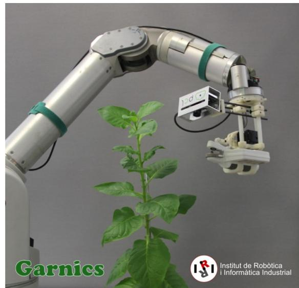
Setups for some projects on robot perception and manipulation recently developed at IRI (CSIC-UPC): a) perceiving and handling clothes [7, 8], b) measuring the chlorophyll of plant leaves for phenotyping [2].
