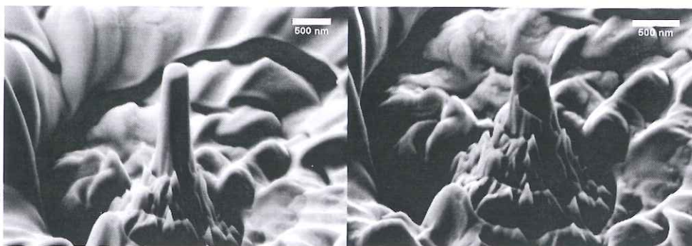
Fig. 2: Degraded 300 nm micro-pillar before and after compression. Grain pull-out during testing is evident in the picture on the right.
