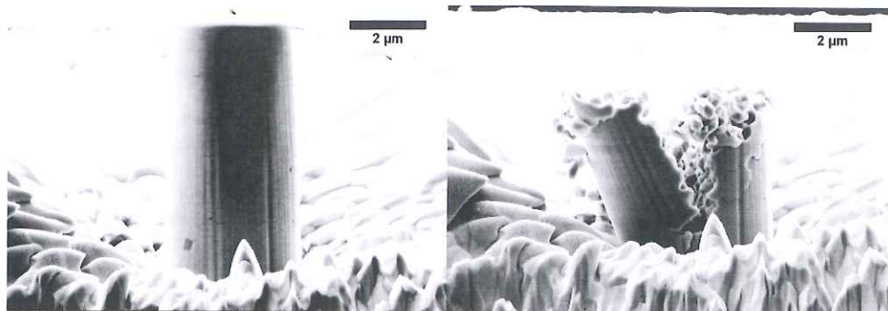
Fig. 1: Degraded 3.3 \mu\text{m} micro-pillar before and after compression. The intergranular character of fracture can be appreciated on the right picture.
