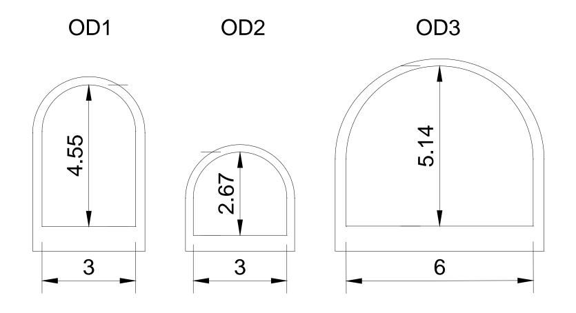
Figure 2. Drains with in situ concrete arches
