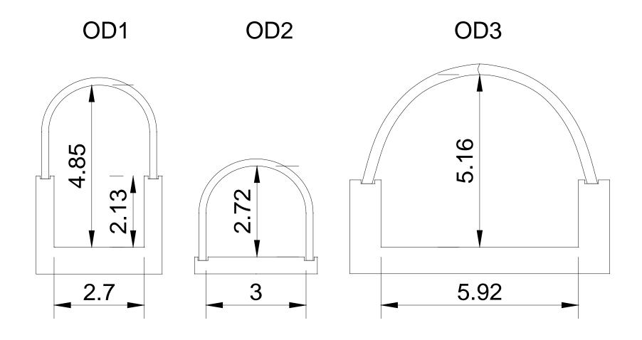
Figure 1. Drains with precast concrete arch
