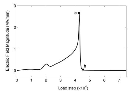
Figure 4: Electric field magnitude  $|\mathbf{E}|$  as a function of the load step obtained at a point in the path of the conducting crack. The crack reaches this point at load step  $\mathbf{a}$  and passes through it at load step  $\mathbf{b}$ .
