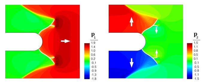
Figure 3: Snapshot of the microstructure evolution in an area near the notch tip under the positive applied electric field with a magnitude of |E| = 1.4 KV/mm. The left and right columns show the horizontal and vertical components of the polarization, respectively. The white lines indicate the position of the cracks (v=0). The domain orientations are indicated with white arrows.
