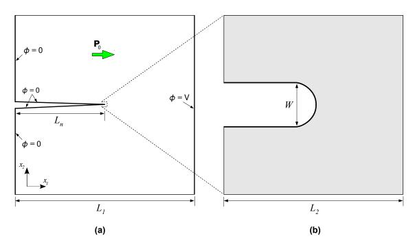
Figure 1: Schematic of the computational domain and loading conditions.
