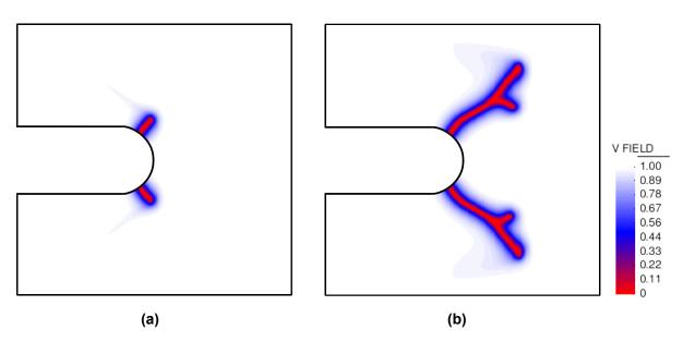
Figure 2: Two snapshots of the fracture evolution: contour plots of the field v under positive electric fields (a) E = 1.12 KV/mm (b) E = 1.4 KV/mm.
